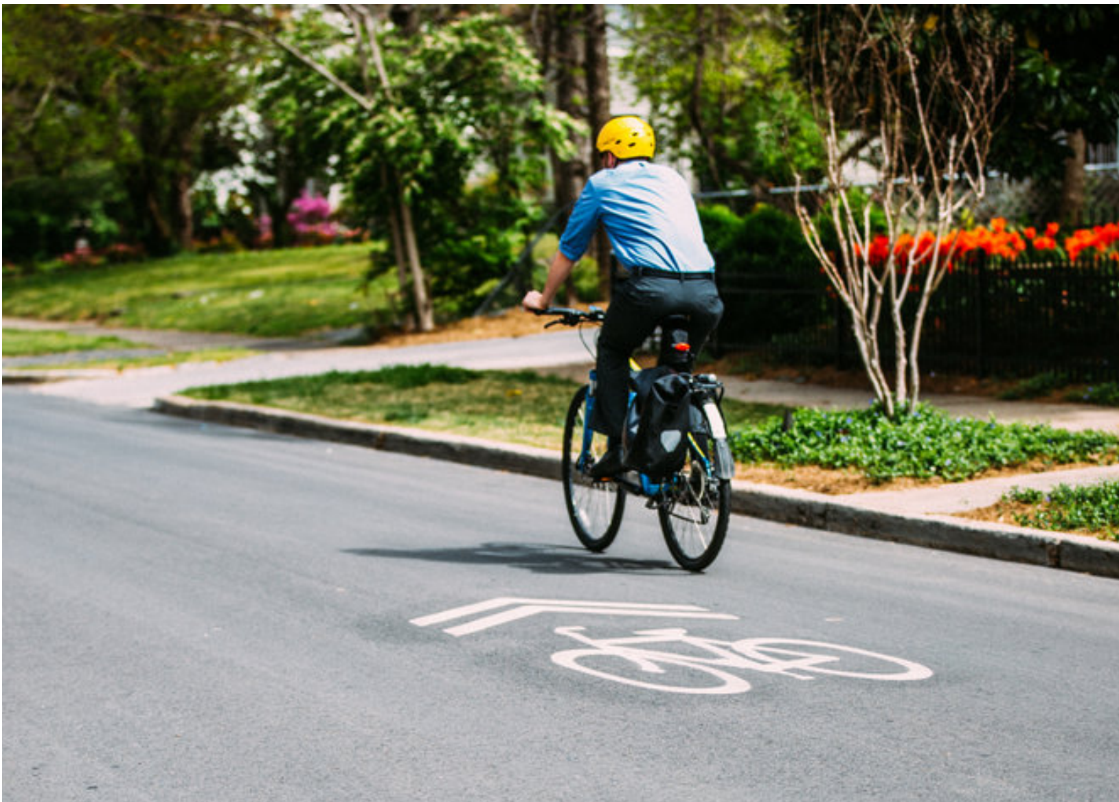
Shared bike lanes are designated by pavement markings called sharrows ; vehicles and bicycles share the travel lane.
