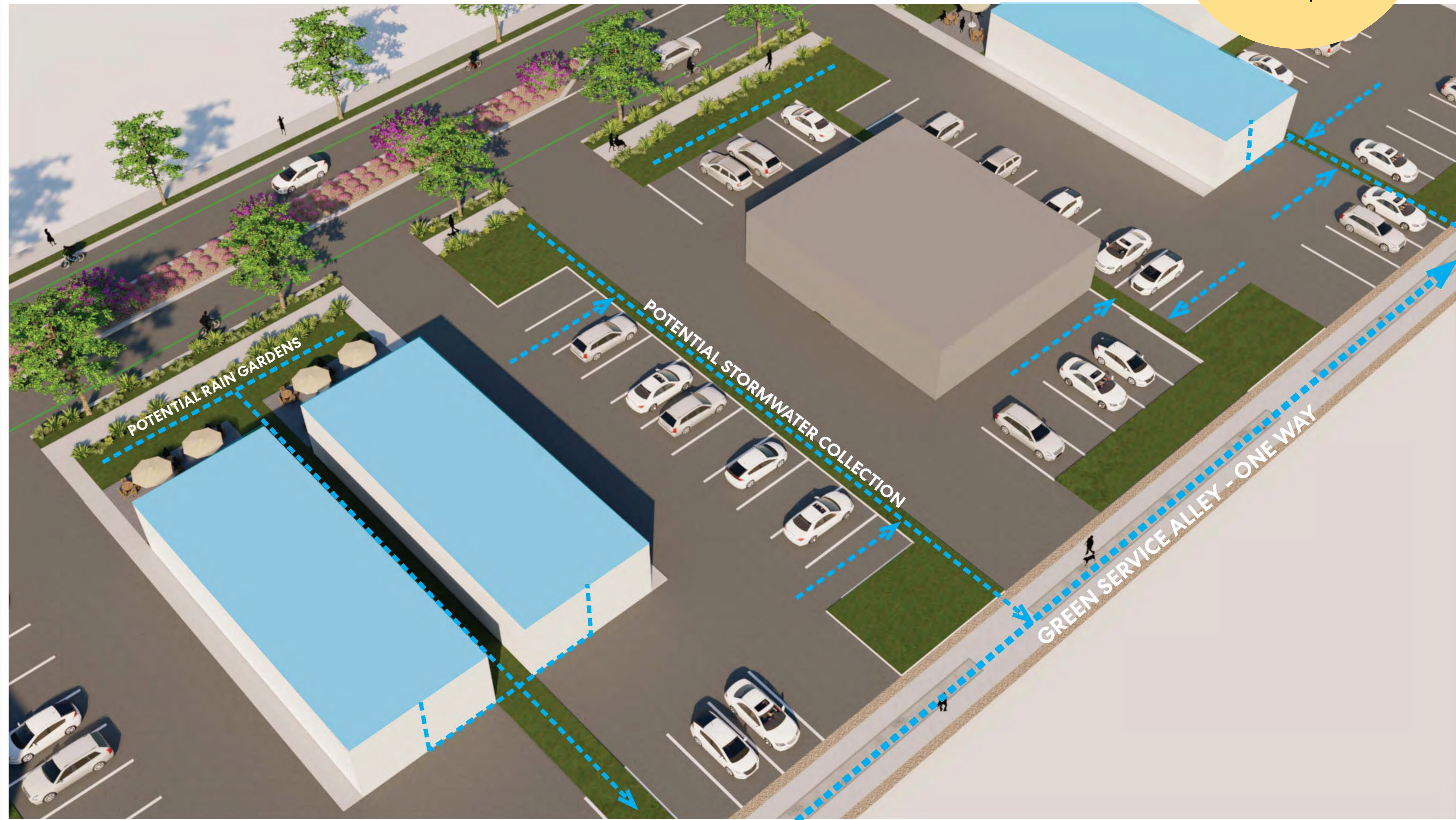
Note the blue lines that illustrate how runoff from building rooftops and parking lots is directed into rain gardens and other planted features that are designed to capture and infiltrate stormwater across the properties.
